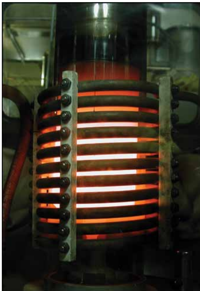
An induction furnace that might be used to heat a plutonium alloy.
